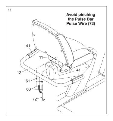
12. Plug the Pulse Bar Pulse Wire (72) into the Frame Pulse Receptacle (75) located in the Left Seat Shield (24).
